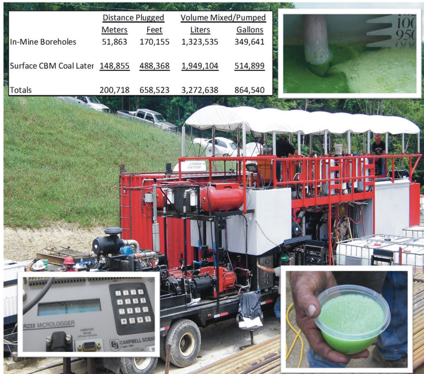
Figure 7. Polymer gel mixing/pumping unit used to plug in-mine boreholes and CBM coal laterals. Plugging with polymer gel summary (top left), mixing polymer gel (top right), monitoring downhole gel pumping pressure (bottom left) and sampling mixed polymer gel per batch (bottom right).
